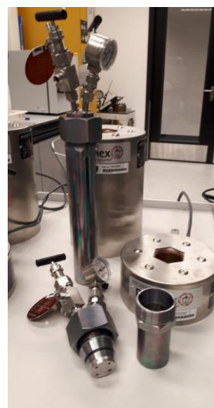
Figure 2. Premex SS reactors (of two different sizes) equipped with pressure/sample inlet/outlet, safety valve and pressure gauge. On the left with Teflon liner and on the right coated with Dursan coating.
